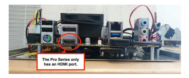
MSI Pro Series motherboards can be identified by the fact that they only have an HDMI port for video output.
