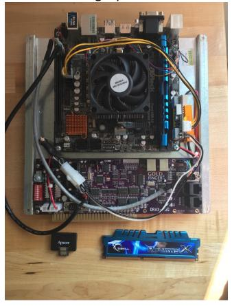
The older MSI boards come with DDR3 RAM and an Apacer hard drive. The hard drive on this board plugs directly into the SATA port.
