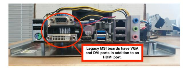
They can be identified by the fact that they have VGA and DVI ports in addition to an HDMI port.
