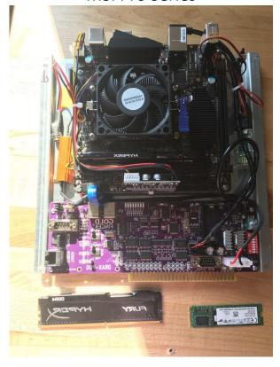
The MSI Pro Series motherboard uses DDR4 RAM and comes with a Plextor hard drive. The hard drives on these boards are mounted on the back of the board.
